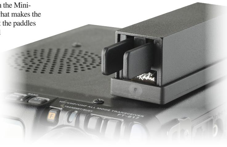
Figure 1 — The Mini-Paddle magnetically attached to my FT-817 transceiver.
